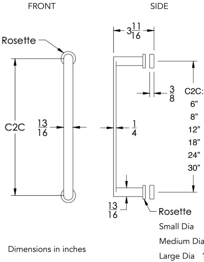
**Installation Notes:** Center to center hole drilling dimension are same as mentioned in column. Diameter of glass hole for installation is 1/2".
